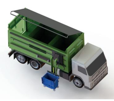
Keox RLH can be installed almost every chassis and it is very customizable. Unit can be splitted for example four different compartments, glass, paper, metal and bio. Keox RHL equipmented with four different compartments is highly cost efficient. Sideways moving elevator can spread or seperate wastes in their own compartments.
